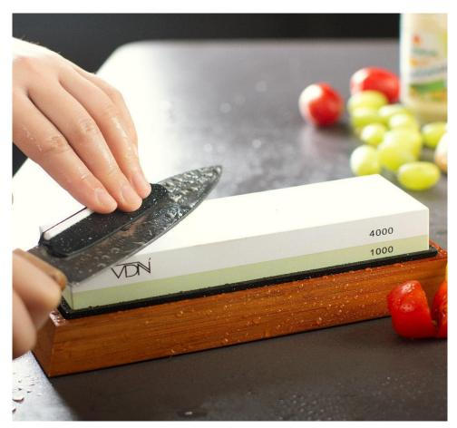
Lay the knife flat on the whetstone and lift the back of the knife with your dominant hand to find the sharpening angle. The exact number of degrees isn't that important. A few degrees more or less don't make a big difference. Instead, it's important to maintain the selected angle throughout the grinding process.
